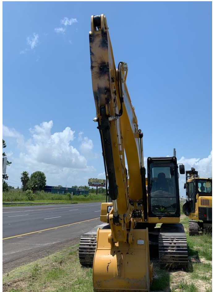
The resulting damage to the arm of the excavator.
