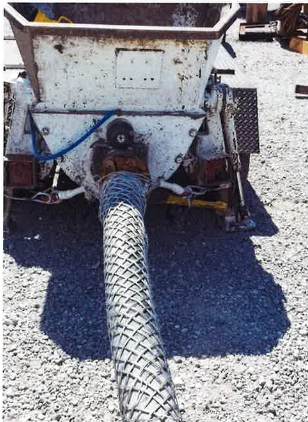
LOOP BAIL GRIP CONNECTING HOSE TO PUMP (CAN BE USED FOR THREAD AND/OR BOLT TYPE CLAMPS)
